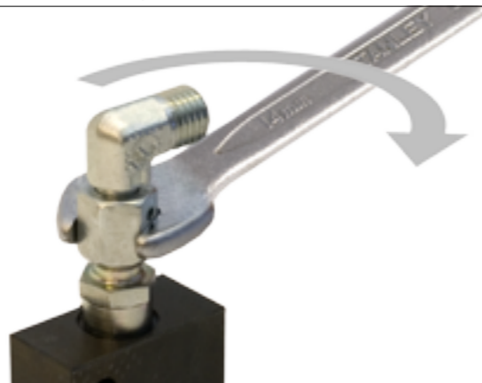
2. Then tighten until sharp increase of resistance, ¼ to ½ turn (if possible use a torque according to next page)
