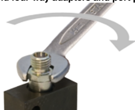
2. Then tighten wrench-tight (if possible apply a torque according to next page)
