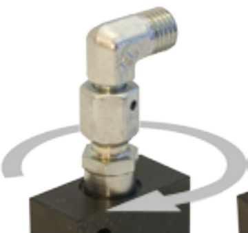
1. Screw on nut until the O-ring is fully compressed (hand-tight)
